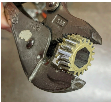
Gear damage (would require a steel replacement or larger gear)
