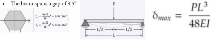
Plugging all of this into the formula we get a maximum beam deflection of 0.0642" which is far above the tolerances we can allow. The hex axles were not going to work.
