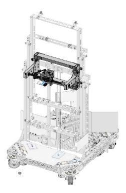
The pivot utilizes a hard stop to allow the intake to rotate between -10 degrees from vertical and 160 degrees from vertical. This ensures that the intake does not hit any of our other mechanisms and expensive components.
