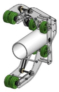
All wheels are powered by one belt system, using spur gears to reverse the belting direction. Both algae and coral intake are run from the same motor.
